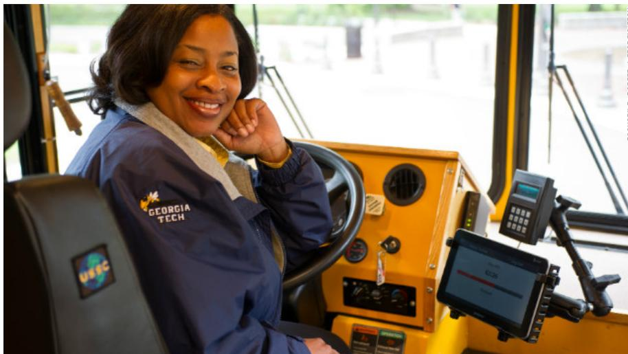
**Figure 1: Android Tablet With Countdown Software Mounted On A Georgia Tech Trolley**
